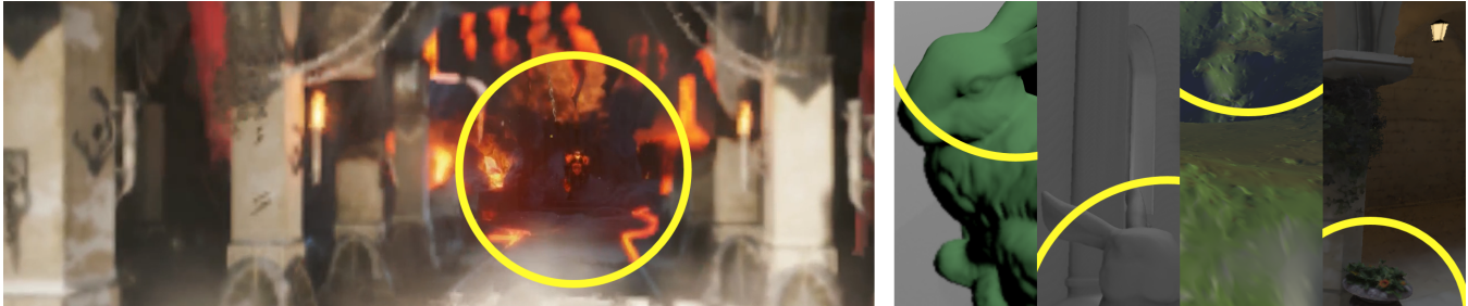
Figure 1: Left: Our foveated resolution method on UE4 and the Elemental Demo ©Epic Games, Inc. Right: Our foveated resolution, ambient occlusion, tessellation, and ray-casting (respectively) methods. Areas outside the circles are rendered in lower detail (peripheral).
